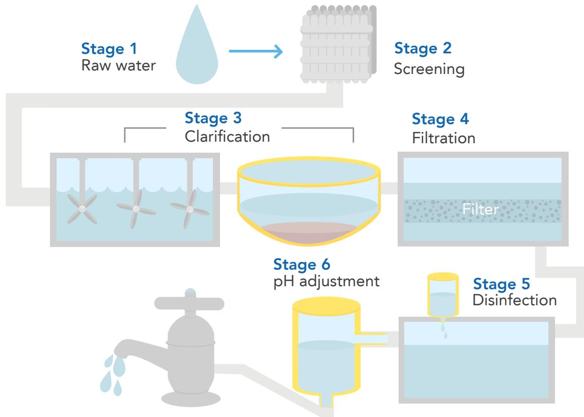
**Stage 1:** Surface water is stored in reservoirs to provide a continuous supply to meet demand throughout the year.
